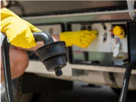
Macerator Sewage Discharge With Manual Disconnect
