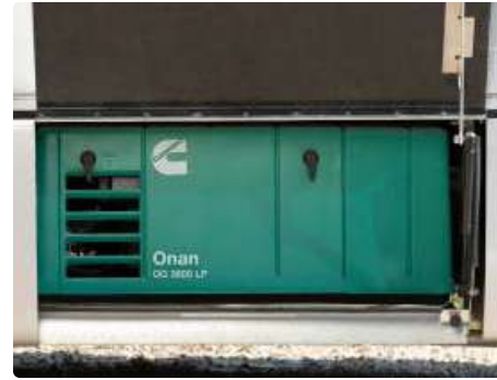
3.6 kW LP Generator With Auto Start and Auto Changeover Switch
